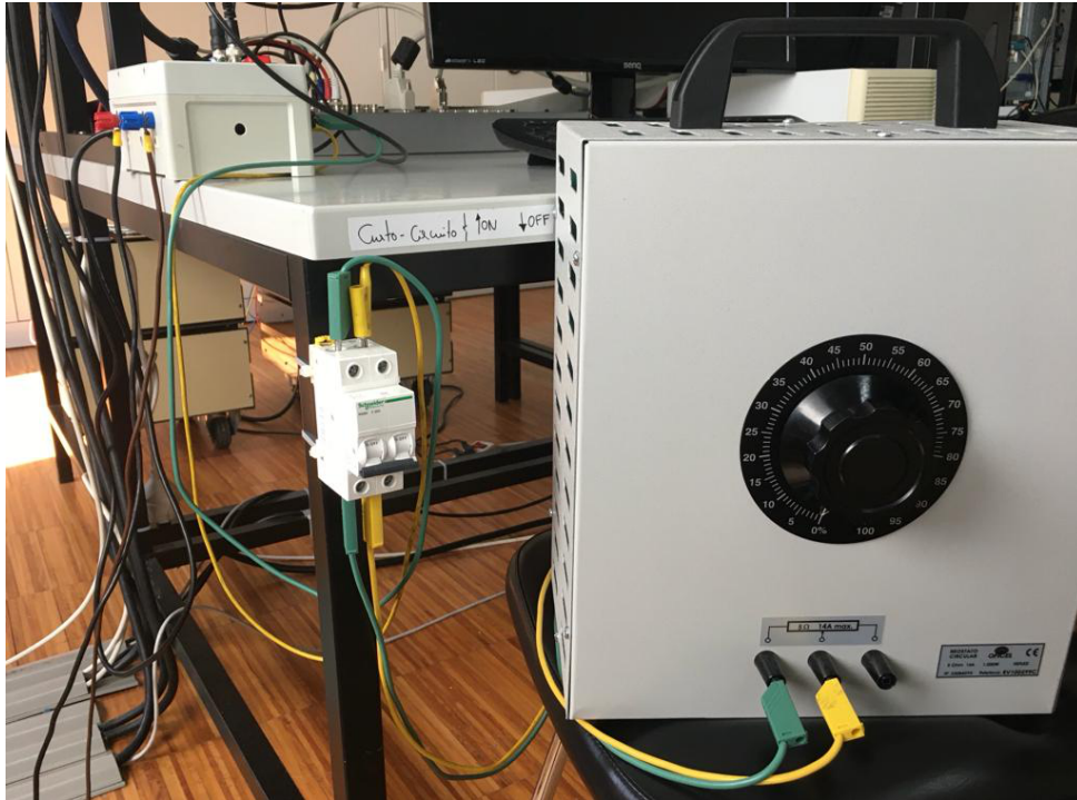
Figure C.6: Additional resistor used in the emulation of interturn short-circuits.
