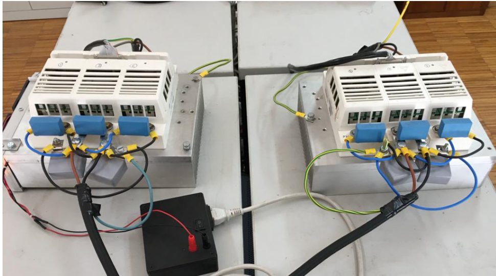
Figure C.3: 2L-VSIs used to power the six-phase PMSM.
